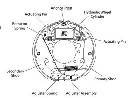
to "wrap around". In essence, the brake has utilized frictional force to help the applying force on both shoes.
