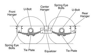
The articulation of this suspension occurs when the rear end of each slipper spring slides against the wear surfaces provided in the rear hangers or equalizers. This suspension is also available in single and multiple axle configurations.
