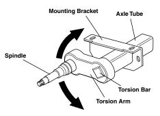
encased in the main structural member of the axle beam.
