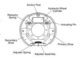
forward direction. Uni-servo brakes are normally used with surge type actuators.
